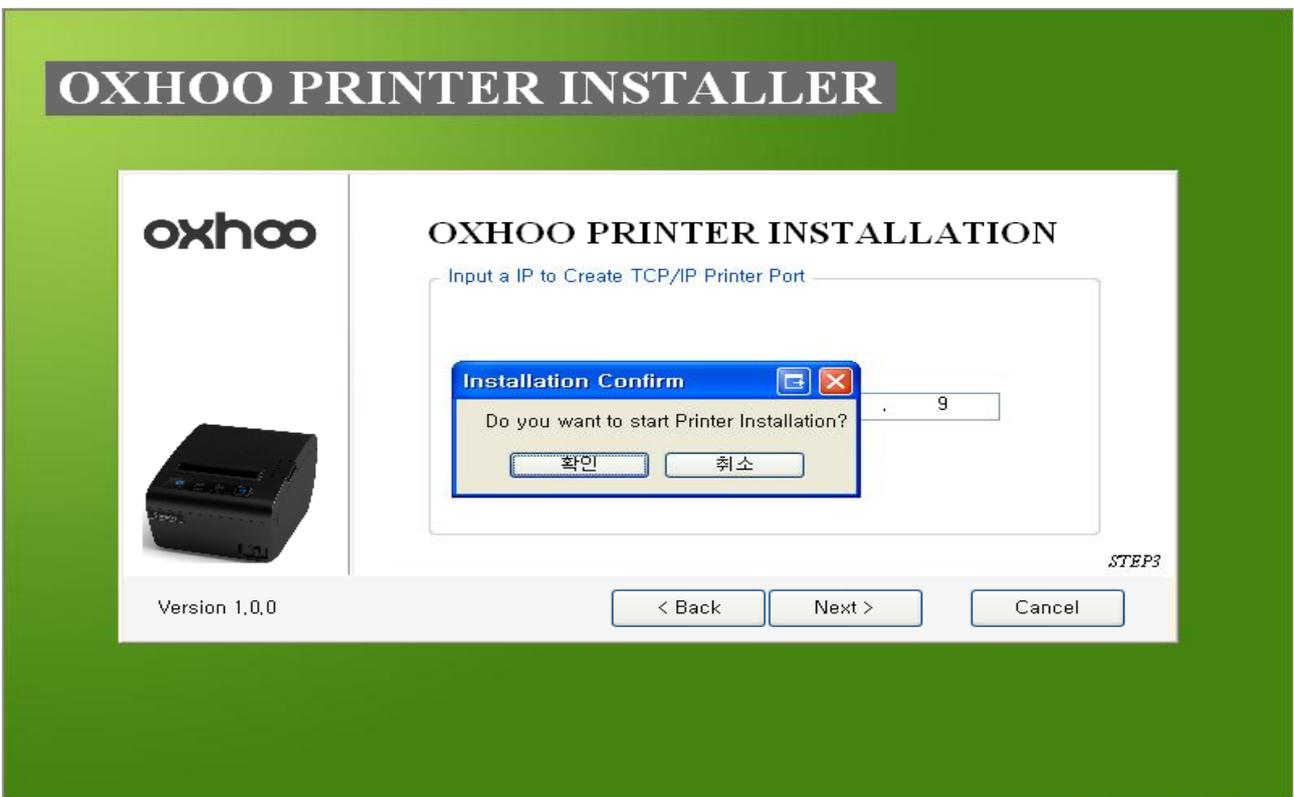
[Pic No.10-3] Start Printer Installation for ETHERNET connection
