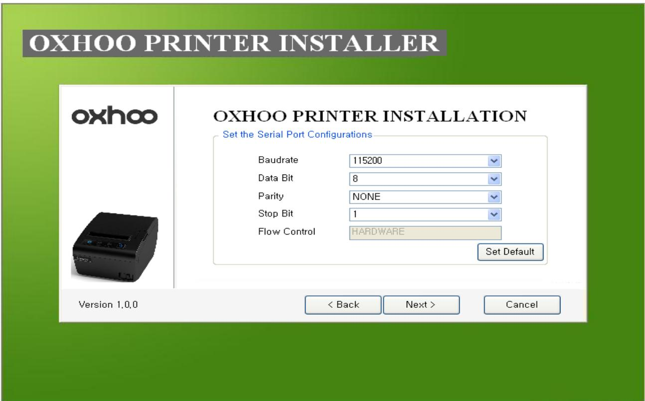
[Pic No.9-2] Set the Serial Port Configurations
