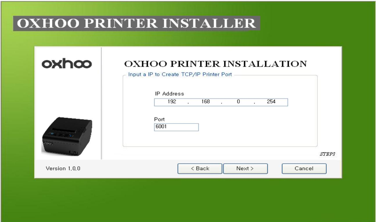
[Pic No.9-3] Create a TCP/IP Printer Port
